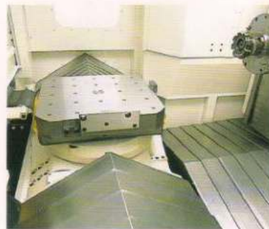
X-Z axes slant waycover
